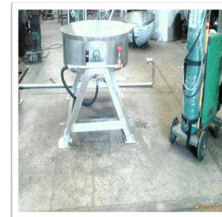
CIP SYSTEM-SKID MOUNTED (600 LTS CAPACITY)
